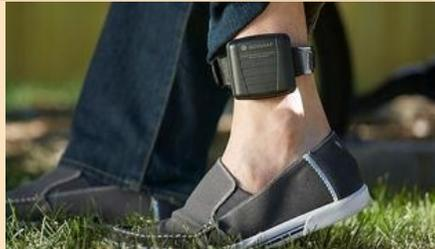
**THE SCRAM CAM ENABLES CONSISTENT ALCOHOL CONSUMPTION MONITORING. IMAGE SOURCE: SCRAM SYSTEMS**
